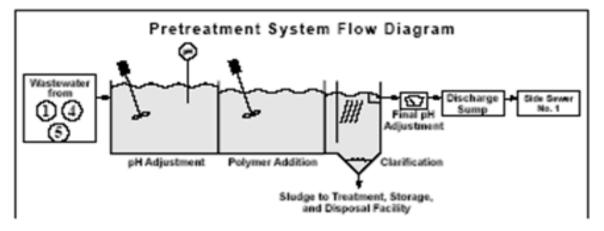
EXAMPLE PRODUCTION/PROCESS SCHEMATIC FLOW DIAGRAM
